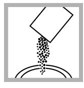
9. Add two 10-mL DPD Free Chlorine Reagent Powder Pillows or two 10-mL DPD Total Chlorine Reagent Powder Pillows to the second sample cell.
