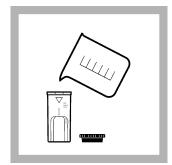
2. Prepare the blank: Fill a 1-cm/10-mL sample cell to the 5-mL mark with sample. Close the sample cell.
