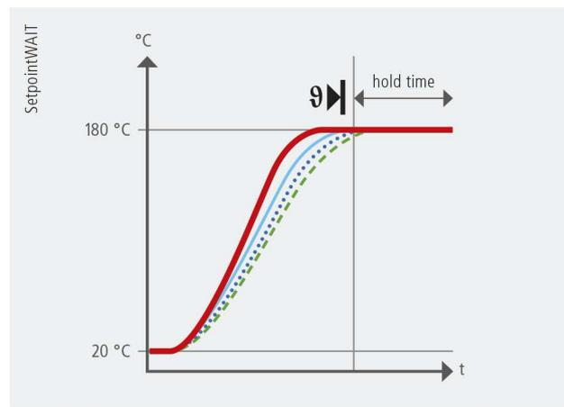
When the SetpointWAIT function is activated, the hold time does not start until the temperature within a very narrow tolerance range is reached at all measuring points
