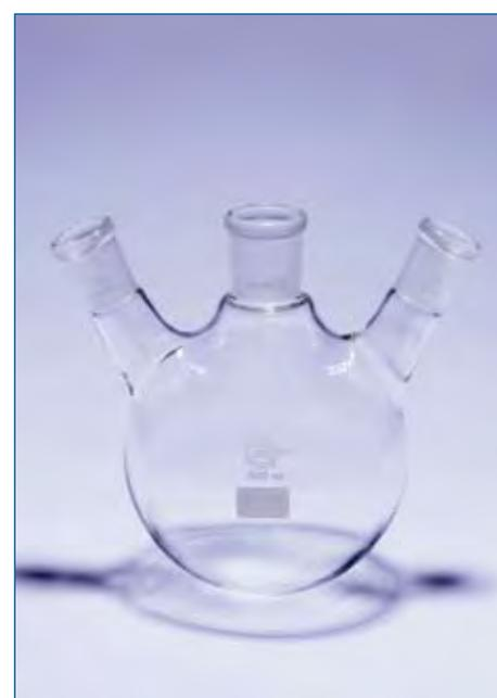
**i** The axes of the side necks meet the axis of the central neck at the bottom of the flask.
