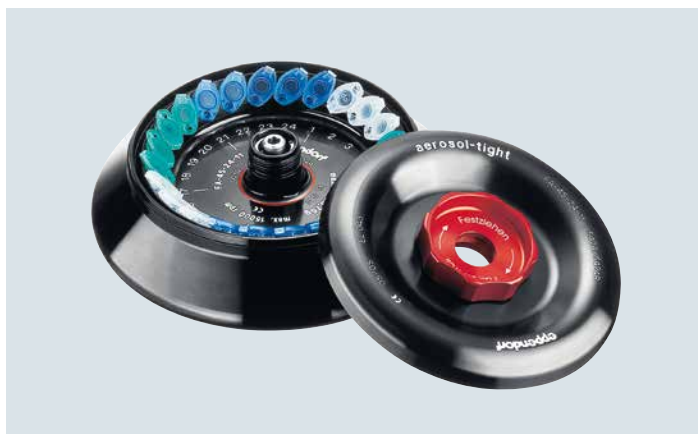
Aerosol-tight rotor for 24 × 1.5/2.0 mL tubes provides speed up to 21,130 \times g/15,000 rpm. (FA-45-24-11; Order no. 5424 702.007).
