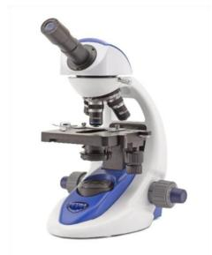
Monocular brightfield microscope, 600x, HC objectives
