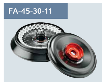
30 × 1.5/2 mL micro tube rotor with aerosol-tight lid for safe centrifugation of hazardous samples. Max. speed 20,800 × g (14,000 rpm).
