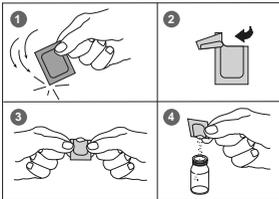
5. Add the contents of **one Vario Manganese Citrate Buffer F10 Powder Pack** straight from the foil to the water sample.
