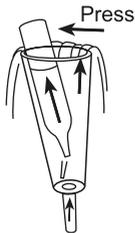
1. Place the blank in the sample chamber. The blank is part of the test kit.
