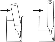
5. Place one Vacu-vial® in the sample container. Snap the tip by pressing the vial against the side of the sample container. The Vacu-vial® breaks at the neck and the vial fills automatically. A small volume of inert gas remains in the Vacu-vial®.
