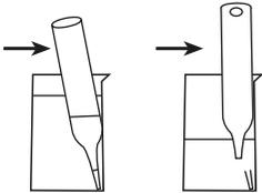
5. Place one Vacu-vial® in the sample container. Snap the tip by pressing the vial against the side of the sample container.
