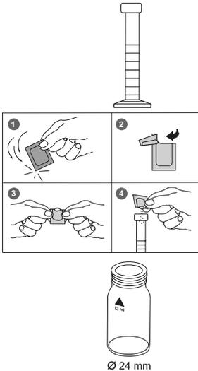
1. Fill a clean Mixing Cylinder (25 ml) with **20 ml of the water sample**.
