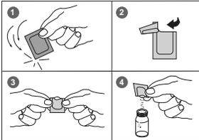
5. Add the contents of **one Vario Ferro F10 Powder Pack** straight from the foil to the water sample.
