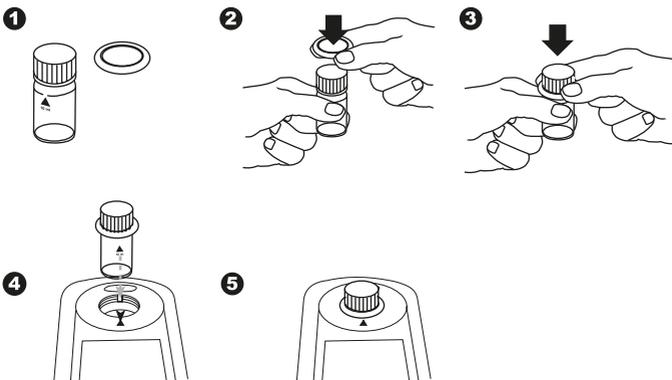
5. Always perform zeroing and test with closed vial cap. Only use cap with sealing ring.
