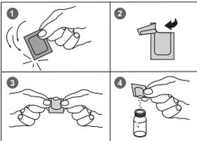
5. Add the contents of **one Chlorine TOTAL-DPD/ F10 Powder Pack** straight from the foil to the water sample (note 5).
