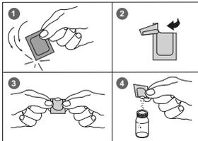
1. Fill a clean vial (10 mm  $\varnothing$ ) with **5 ml of the water sample**, close tightly with the cap.
