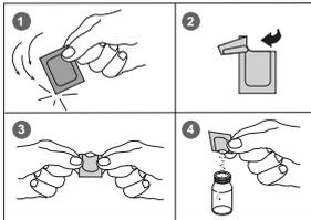
1. **Open two TN Hydroxide HR digestion vials** and add the contents of **one Vario TN Persulfate Rgt. Powder Pack** (Note 2, 3).
