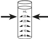
4. Fill the sample container to the 25 ml mark with the water sample.
