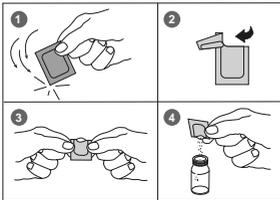
5. Add the contents of **two Chlorine Free-DPD/ F10 Powder Pack** straight from the foil into the water sample.
