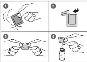
1. **Open two TN Hydroxide LR digestion vials** and add the contents of **one Vario TN Persulfate Rgt. Powder Pack** (Note 2, 3).
