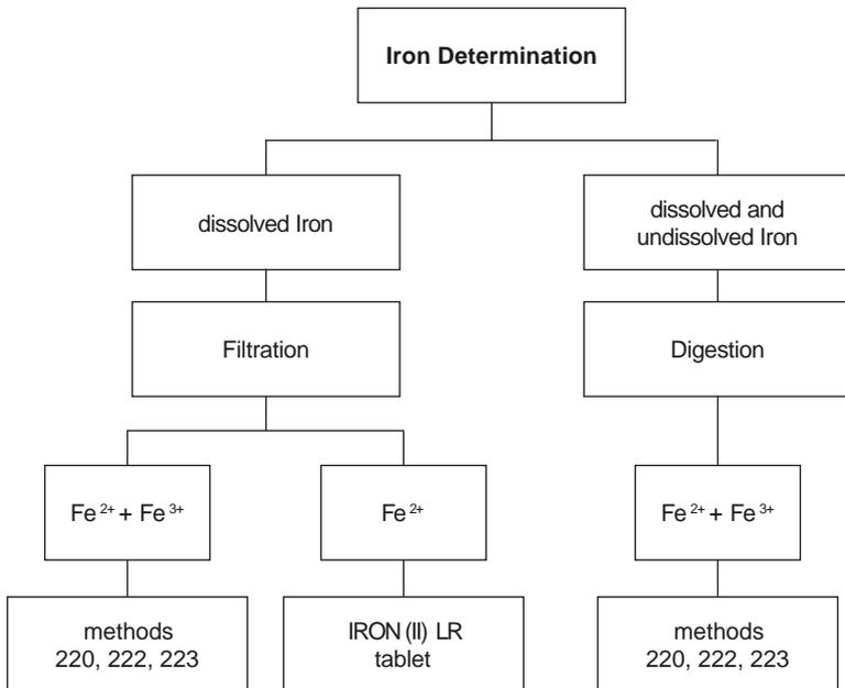
**Digestion procedure** for the determination of total dissolved and undissolved iron.
