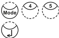
If the test result is displayed press [MODE], [Shift] + [4] [5] keys and confirm with [↵] key.
