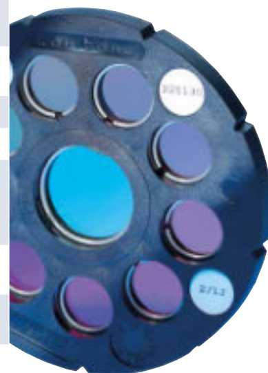
Test disc with colour-stable glassstandards
