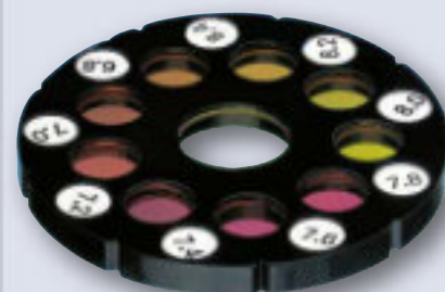
Test disc with colour stable glassstandards
