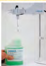
Step 2: Gently squeeze the bottle to fill the calibration chamber with standard solution.
