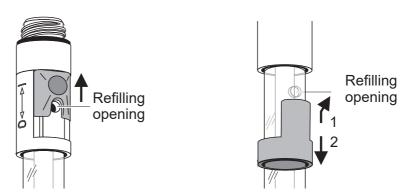
• Remove the watering cap from the electrode tip. Possible salt deposits in
