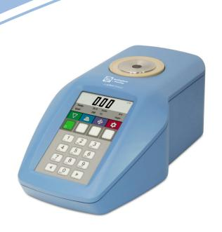
RFM700 series refractometers are robust, low cost, fully automatic instruments that are ideally suited to the food, sugar and beverage industries but can also be used in many other non-food applications where temperature control is not required.
