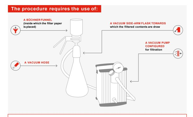
The mixture to be filtered is poured into the funnel. The latter is fitted into the flask, with a rubber conical seal ensuring an air-tight connection of the two elements. When the vacuum pump, which is connected through tubing to the side spout of the flask, is turned on, vacuum pulls the mixture down through the filter paper. The filtrate is captured in the flask, while the solids are collected on top of the filter paper.
