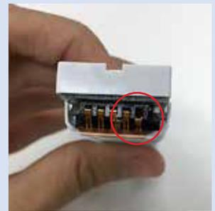
Figure 3.1: Bent pins inside the meter
