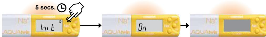
5. Press MEAS and ON/OFF buttons simultaneously for 3 seconds.
