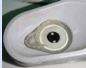
Figure 1.1: KCl salts build-up on the sensors is a normal occurrence
