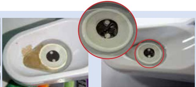
Figure 1.2: Sensor with cracked or broken membrane
