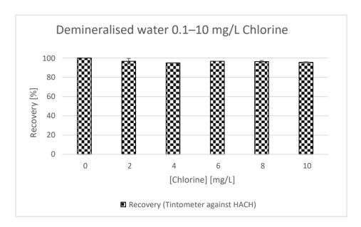
Figure 17: Recovery rates of total chlorine in demineralised water with different chlorine concentrations measured with "Tintometer total chlorine DPD/F25" in comparison to "HACH DPD Total Chlorine Reagent Powder Pillows, 25 mL"
