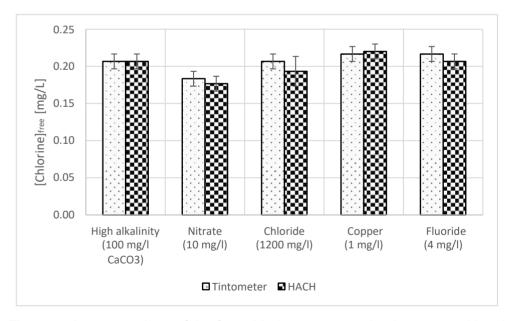
Figure 5: Average values of the free chlorine concentration in waters with select contents measured with "Tintometer Chlorine free DPD/F10" / "HACH DPD Free Chlorine Reagent Powder Pillows, 10 mL"
