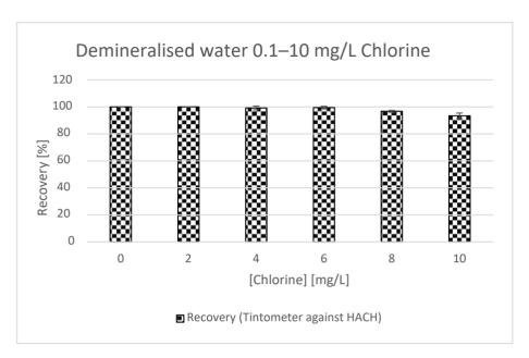
Figure 7: Recovery rates of the free chlorine in demineralised water with different chlorine concentrations measured with "Tintometer Chlorine free DPD/F25" in comparison to "HACH DPD Free Chlorine Reagent Powder Pillows, 25 mL"
