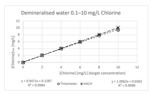
Figure 2: Recovery functions: Free chlorine in demineralised water (0.1–10 mg/L);
