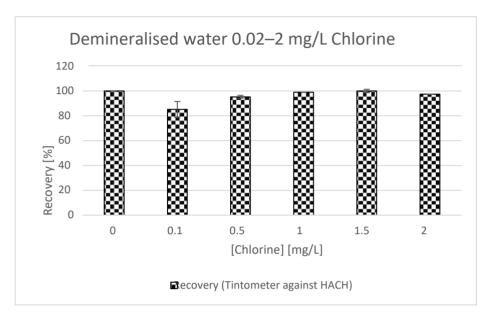
Figure 6: Recovery rates of the free chlorine in demineralised water with different chlorine concentrations measured with "Tintometer Chlorine free DPD/F10" in comparison to "HACH DPD Free Chlorine Reagent Powder Pillows, 10 mL"
