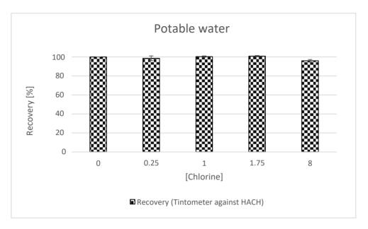
Figure 19: Recovery rates of the total chlorine in potable water with different chlorine concentrations measured with "Tintometer total chlorine DPD/F10 and F25" / "HACH DPD Total Chlorine Reagent Powder Pillows, 10 mL and 25 mL"
