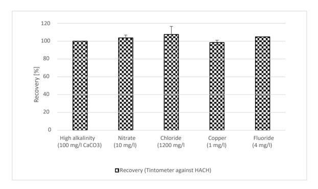
Figure 10: Recovery rates of free chlorine in waters with select contents measured with "Tintometer Chlorine free DPD/F10" in comparison to "HACH DPD Free Chlorine Reagent Powder Pillows, 10 mL" with a free chlorine concentration of 0.25 mg/L
