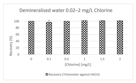
Figure 16: Recovery rates of total chlorine in demineralised water with different chlorine concentrations measured with "Tintometer total chlorine DPD/F10" in comparison to "HACH DPD Total Chlorine Reagent Powder Pillows, 10 mL"
