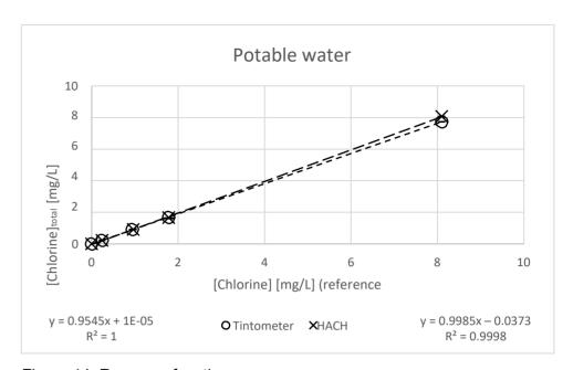
Figure 14: Recovery functions: Total chlorine in potable water (0.25–8 mg/L);
