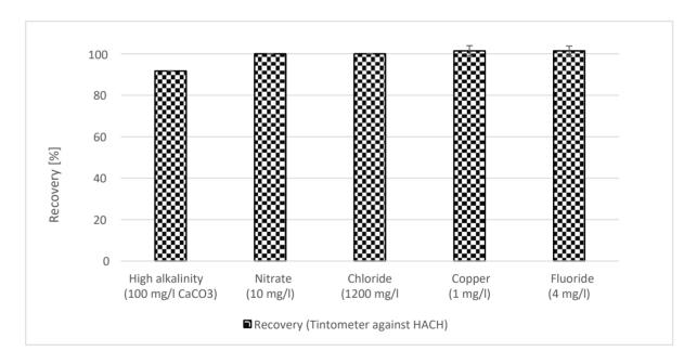
Figure 20: Recovery rates of total chlorine in waters with select contents measured with "Tintometer total chlorine DPD/F10" in comparison to "HACH DPD Total Chlorine Reagent Powder Pillows, 10 mL" with a free chlorine concentration of 0.25 mg/L
