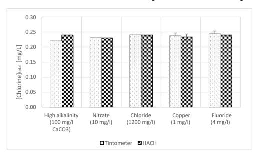
Figure 15: Average values of the total chlorine concentration in waters with select contents measured with "Tintometer Chlorine total DPD/F10" / "HACH DPD Total Chlorine Reagent Powder Pillows, 10 mL"
