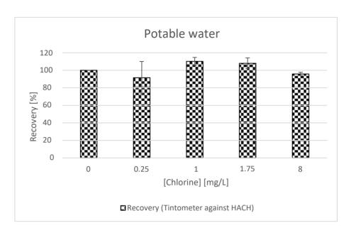
Figure 9: Recovery rates of free chlorine in potable water with different chlorine concentrations measured with "Tintometer Chlorine free DPD/F10 and F25" / "HACH DPD Free Chlorine Reagent Powder Pillows, 10 mL and 25 mL"
