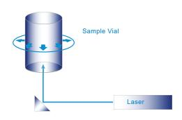
Figure 1— The 360° x 90° Detection technology directs a beam of light into your sample, which is then read at 360 degrees of detection for hightly accurate and repeatable measurements.
