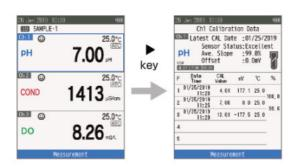
In the focused ID of the measurement mode, the sensor condition of each sensors can be viewed by pressing the  $\blacktriangleright$  key.
