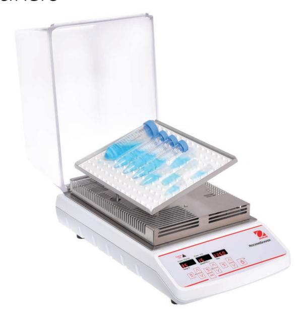
OHAUS Incubating Rocking and Waving Shakers are designed to incubate samples from 5°C above ambient to 65°C to provide accurate and repeatable results. Rocking shakers provide a see-saw like motion, while waving shakers offer a smooth, low-foaming three-dimensional "wave" motion. All models feature LED displays with touchpad controls. Both models include safety features that protect both the user and samples.
