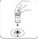
Remove the vial from the sample chamber.
