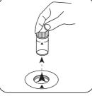
Remove the vial from the sample chamber.
