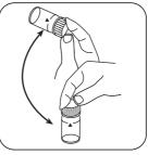
Dissolve tablet(s) by inverting.
