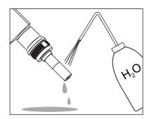
Rinse the sensor head with deionized water.
