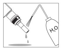
Rinse the sensor head with deionized water.
