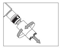
Pull off the stirring paddle and screw off the membrane head.
