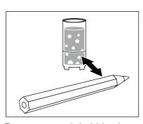
Remove any air bubbles by carefully tapping the membrane cap. Additionally, you can prevent air bubbles by throwing the first filling away and refilling the membrane cap.
