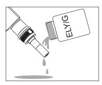
Rinse the sensor head with electrolyte solution.
