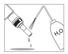
Rinse the sensor head with deionized water.
