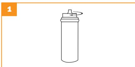
Direct the valve away from you, press it down and turn it clockwise until it is locked.
